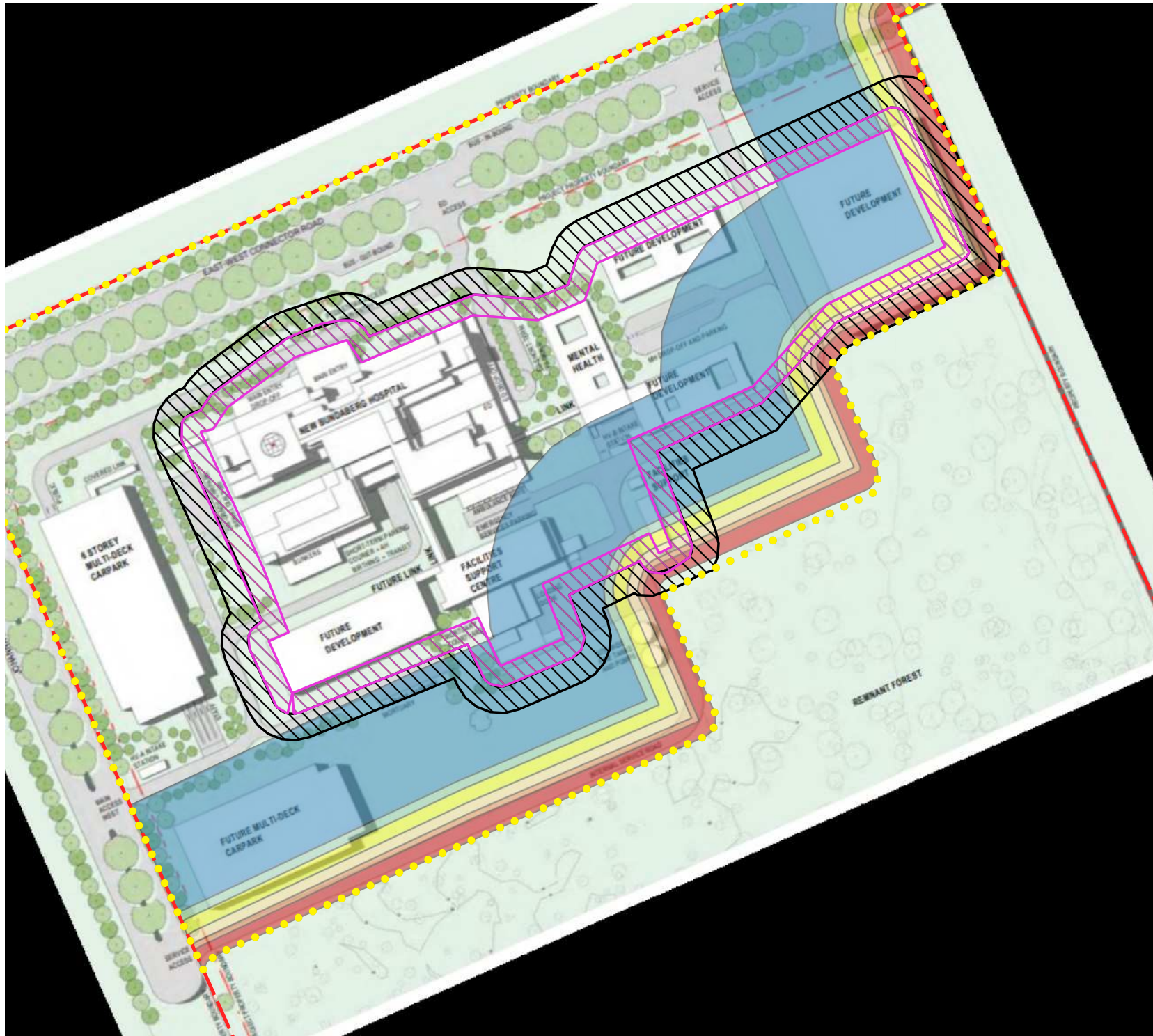
Figure 7: Bushfire Attack level And Asset Protection Zone
