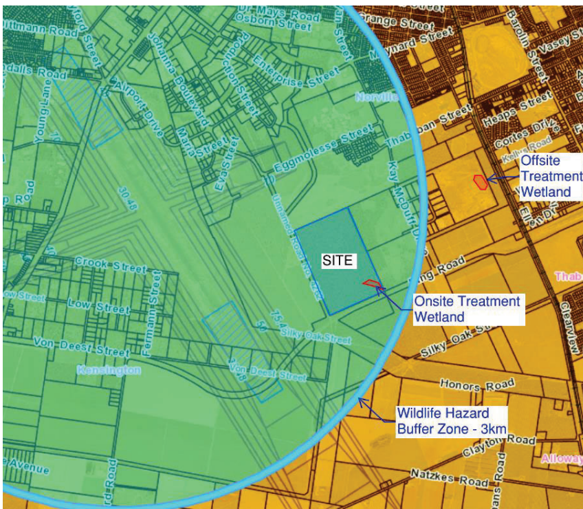
Figure 7-2: SPP Runway Buffer Overlay
